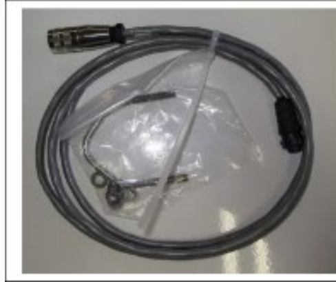
Temperature probe installation. Connect the silver connector of the temperature cable to the silver connection on the bottom of the sensor
