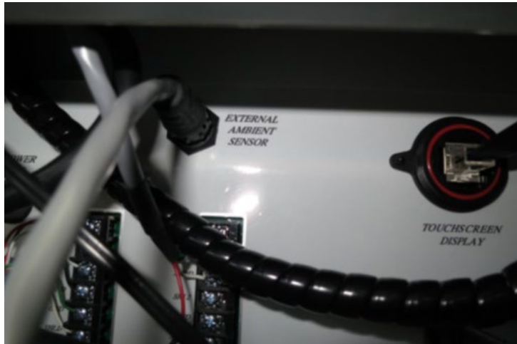
Route the sensor cable to the back of the enclosure and attach it to the connection labeled as EXTERNAL AMBIENT SENSOR
