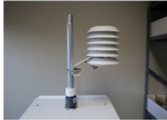
Temperature probe installation. Connect the silver connector of the temperature cable to the silver connection on the bottom of the sensor
