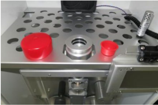
Downtube seats into the inlet receiver collar O-rings
