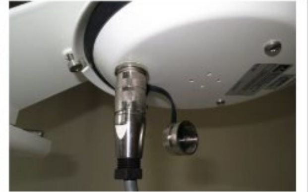
Temperature probe installation. Connect the silver connector of the temperature cable to the silver connection on the bottom of the sensor
